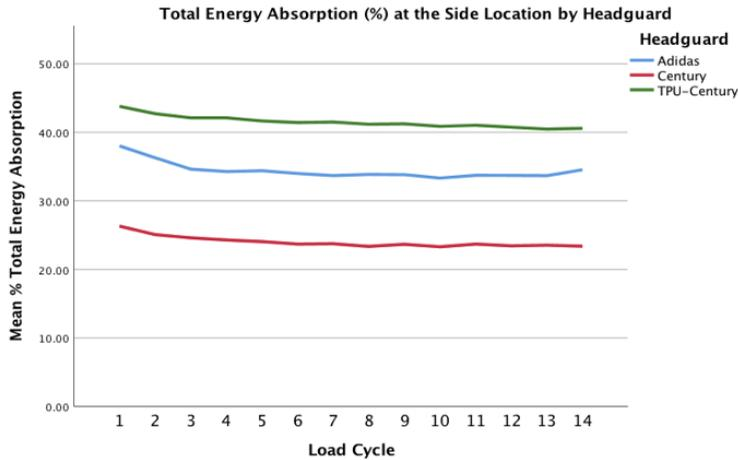
When separating the total energy into compressive and shear energies, the TPU-Century→ Drive had the highest mean percentage of absorbed compressive energy (M=48.48%), when compared to the Adidas→ (M=40.10%), and Century→ Drive (M=28.66%) headgear. Similarly, for the shear energy, the TPU-Century→ Drive absorbed the highest percentage of shear energy (M=29.15%), when compared to the Adidas→ headguard (M=22.48%), and the Century→ Drive headgear (M=13.51%).
