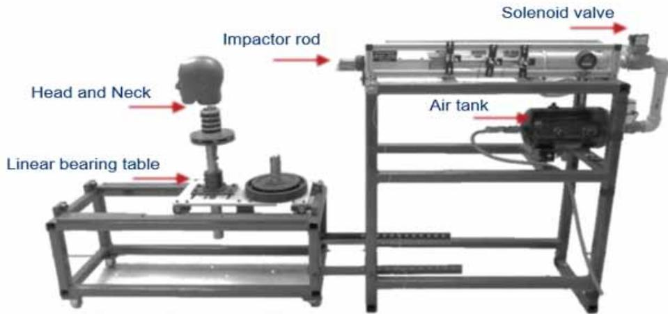
2019) headform, which was attached to a mechanical neckform as depicted in Figure 3. The surrogate headform and mechanical neck form represented the 50<sup>th</sup> percentile of a human head and neck.
